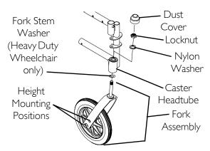
FIGURE 8.1 Installing/Replacing/Adjusting Front Casters and Forks
